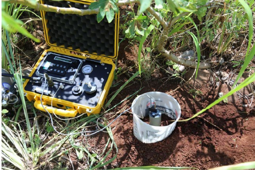
Photo 4-2: The Cohesive Strength Meter test deployed at a fill terrace in Wahikuli
